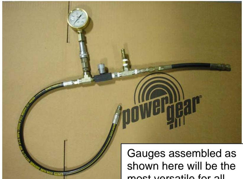
Gauges assembled as shown here will be the most versatile for all applications.
