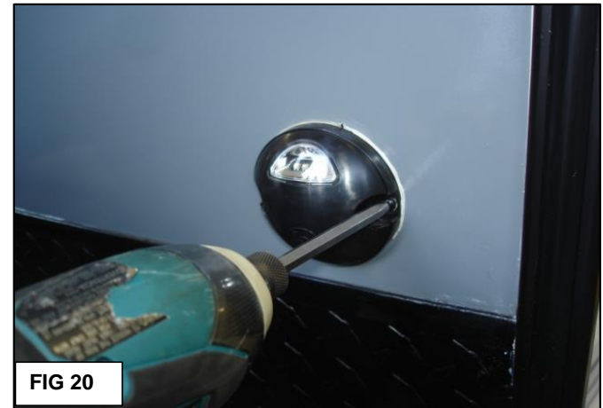
Fig 20: Remove two screws on the Sway Command light pod on the front of the trailer. Remove the pod, and unplug the connector from behind the light pod.
