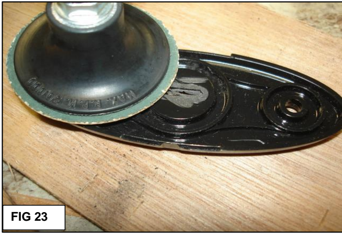
13 Fig 23: Protrusion has been removed with the die grinder.
