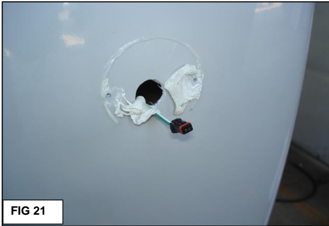
12 Fig 21: Clean the caulking from around the pod location using isopropyl alcohol and a clean rag. Wrap electrical tape around the connector, and push it into the hole, it will not be re-used.
