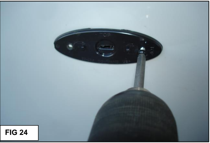
Fig 24: Place the reflector base over the large hole, and secure it with two #8 x 1" pan head screws. A small level may be used to ensure the base is installed straight. A second reflector will be installed on the left side of the RV. Measure the approximate center location of the reflector base just installed, from the side and from the bottom of the RV. Make a mark on the left side of the RV at those same measurements and install a second reflector base with 2 screws. Check the reflector with the level to make sure it is straight.
