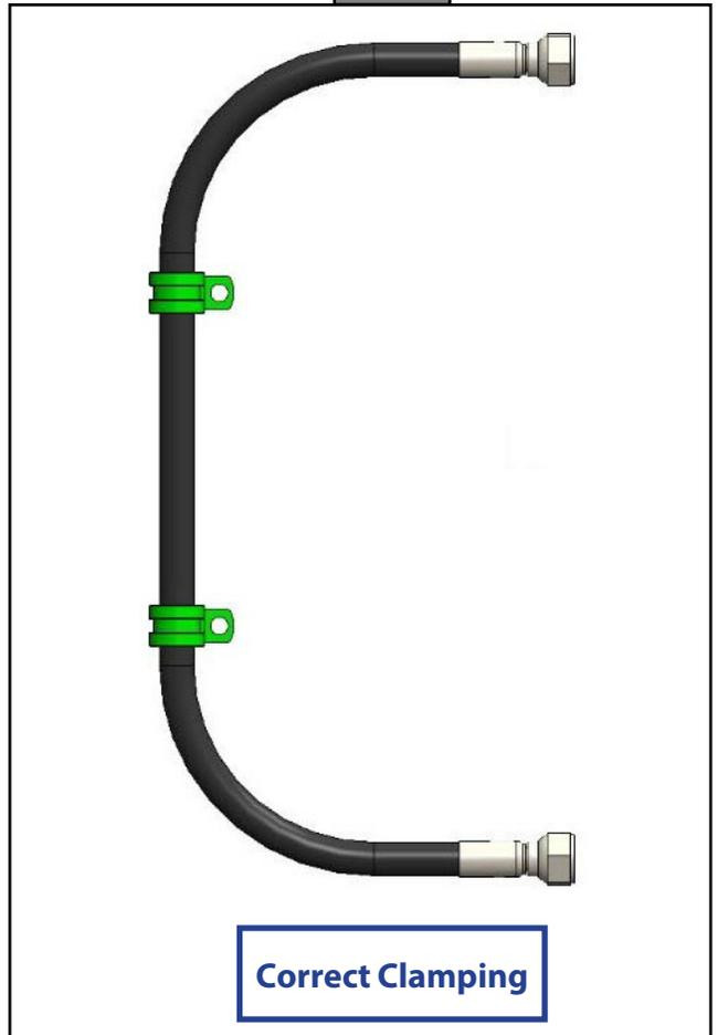
**NOTE:** Clamps should fit snugly to limit movement, but not tight enough to cause damage to the hose. Ensure that there is sufficient slack on each side of the clamp to allow for contraction and expansion of the hose.
