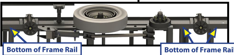
5. Place properly-rated jack stands under the chassis as an added safety measure.
