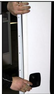
While holding the door closed with one hand, put pressure on the door in the latch area (Fig. 3).
