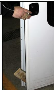
Place the 2x4 at a 45-degree angle between the entry door and the frame down at the threshold. Close the entry door enough to hold the 2x4 in place (Fig. 4). Repeat Fig. 3 and note the "Caution".
