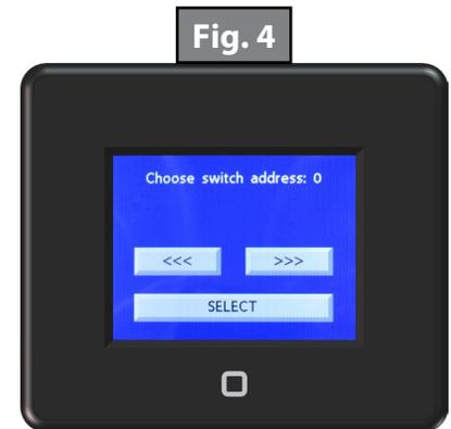
3. Select the desired names to correlate with the functions of the Multifunction board by scrolling through the options with the left and right arrows. After each name is selected press SELECT to advance to the next function. If there is a function(s) not used select NONE (Fig. 5).
