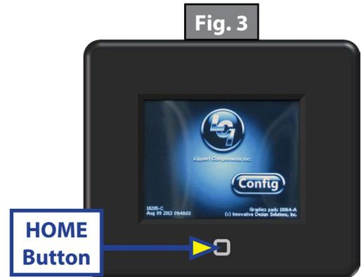
2. The first menu is to program the LINC2CAN switch address (0-15). Each linc touch panel on the bus should have a different address. Scroll to the desired address and press SELECT. The best practice is to start at 0 and continue from there for the rest of the switches. Select the desired address and press SELECT (Fig. 4).
