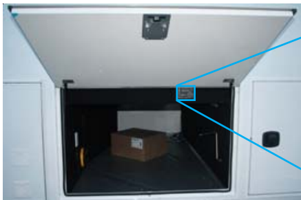
FIG. 3 - Storage Compartment - Note location of touch panel.
